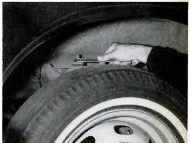
TOP END of front shock absorber on this car can be reached in wheel well without removing the wheel
